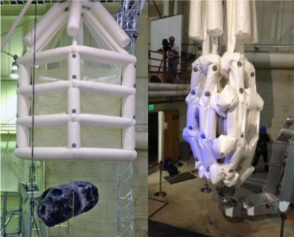
**Figure 2: The ARRMA asteroid capture testbed, showing before and after a demonstration of the inflatable system. On the left the asteroid (below) is being approached, and on the right the asteroid has been captured and the system is deflated and constricted to hold it.**
