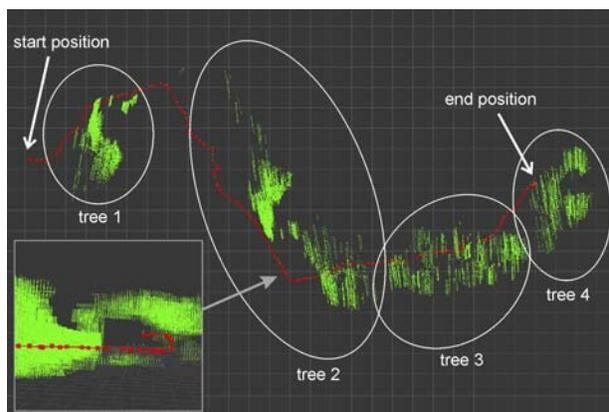
**Figure 7: Data from a test of stereo vision based collision avoidance of a quadrotor helicopter flying between trees. See text for details.**
