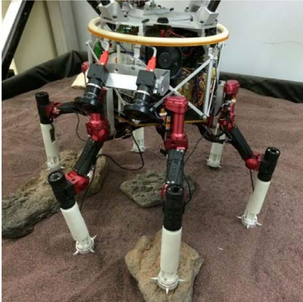
**Figure 5: The SmalBoSSE limbed robot in its test bed with active gravity compensation.**
