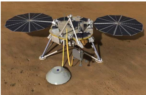
**Figure 1: Artist's rendering of the InSight lander on the surface of Mars. The IDA is shown deploying the HP3, while the SEIS is already deployed and covered by the WTS.**
